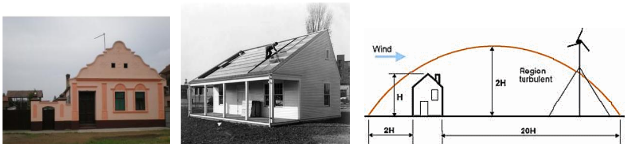
Fig. 4: The concept of urban batteries in Vojvodina. The whole longitudinal side of a housing lot is always facing the sun. Housing lots have appropriate spatial and functional configuration for installing small wind turbines. Source: Simic, I: URBAN BATTERIES - The energy potential of small urban and rural settlements in the region of Vojvodina , IAS-STs Conference 2011, Graz
